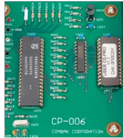
Conventional: The control unit with program and computer chip for the Philips drive is the only thing conventional in the Reimyo CDT-777
