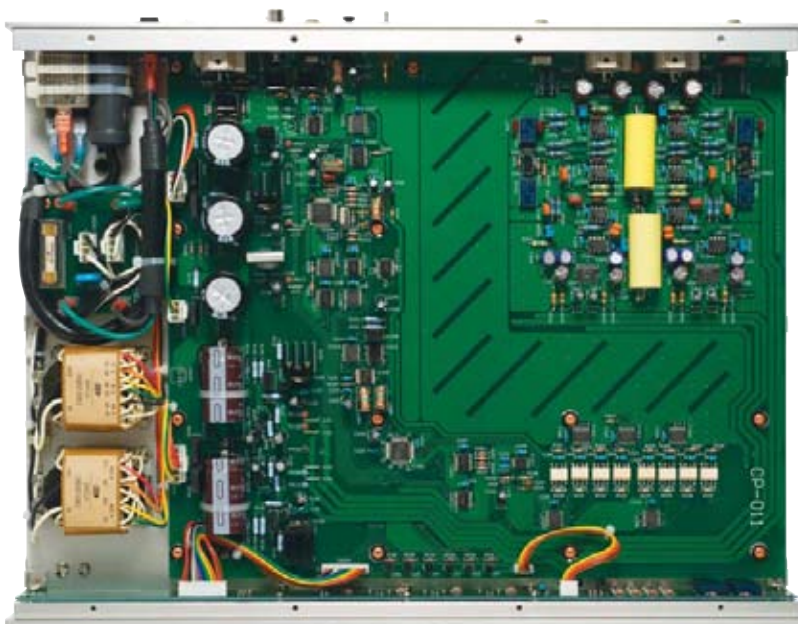
Note the considerable (intentional) physical distance among the power supply, the all-digital section (at left) and the analog output circuits (upper right)
